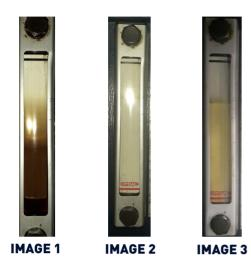
The first image shows the machine sight glass before the clean: the heavy build-up of varnish is clearly visible. After running Milliclean 1000T through the system for 48 hours, the varnish build-up was removed, as can be seen in the second image. The third image shows the machine sight glass refilled with the new, filtered oil.
